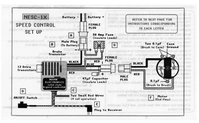
A-On the speed control, solder a female plug on the wires to the motor and a male plug on the wires to the battery. USING THE SAME TYPE OF PLUGS FOR BOTH CONNECTORS VOIDS THE WARRANTY. Hint: Set up your car so you can plug the motor directly into the battery.
