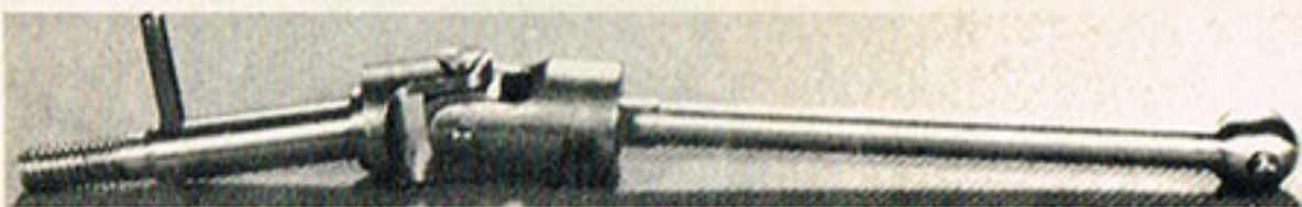
One option is the full length universal jointed drive shaft, which replaces both the shafts supplied in the kit and the standard axles.
