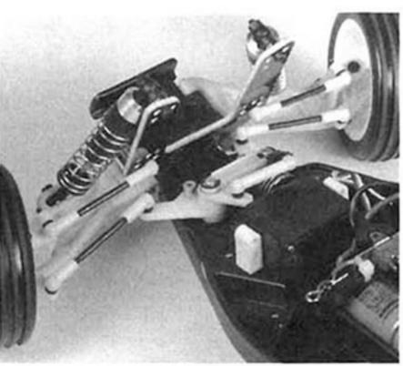
the compact steering linkage is visible. You can also notice the lack of turnbuckles. I had to use with my ESC.
