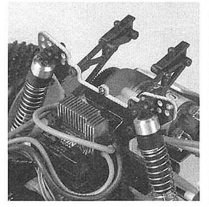
The ESC (if it's not too big) mounts on a shelf above the battery. The adjustable wing mounts are sturdy and stay locked in position even after a crash.
