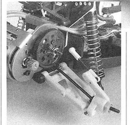
Above: the front suspension has all the adjustments you need, although changing caster requires optional parts. The plastic shocks worked well but tended to stick after they had sat awhile. Left: the rear suspension offers plenty of adjustments, including toe-in options of 1.5, 3 and 5 degrees. If you build the kit, notice that the pivot ball uses the lower hole in the rear hub.
