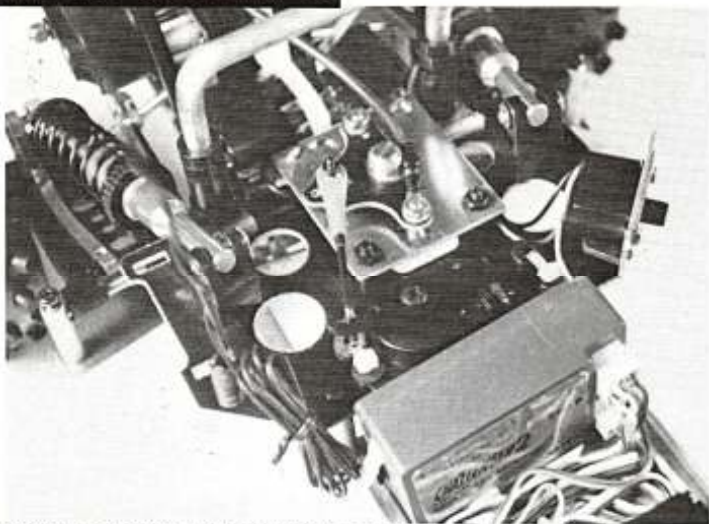
Completed installation of throttle control. Separate receiver battery pack is required. Note receiver is double-stick taped to servo.
