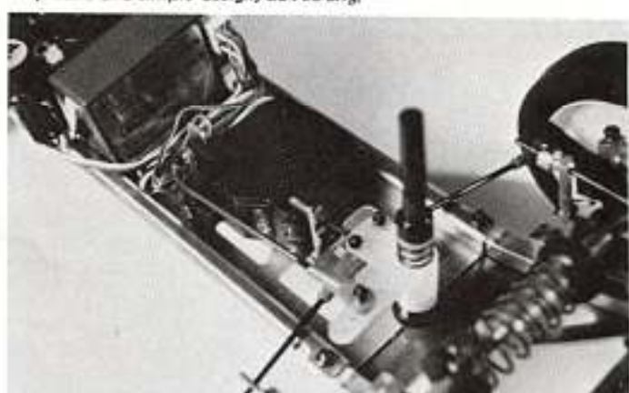
Challenger receiver is a little too wide to fit between rails, must be tilted as shown to clear throttle arm.
