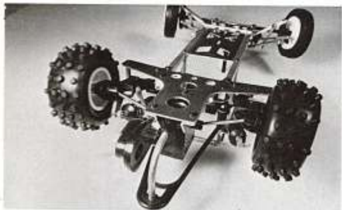
Underside view of assembled chassis as it comes from manufacturer. Side rails are aluminum bar stock.
