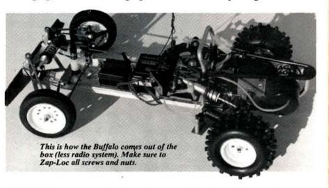
Turbo Pack battery also from Texson. I already had the tools necessary to do what little assembly there is, but if you don't have them, you'll need a Phillips-head screwdriver, needle-nose pliers. scissors, a hobby knife, a thread-locking compound such as Pacer's\* Zap-Loc, an instant adhesive such as Pacer's Zap-Ca, acrylic paint, and a brush.
