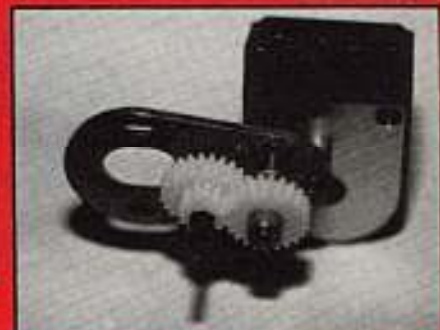
Close up of the gearbox showing two reduction gears and the motor mounting position.
