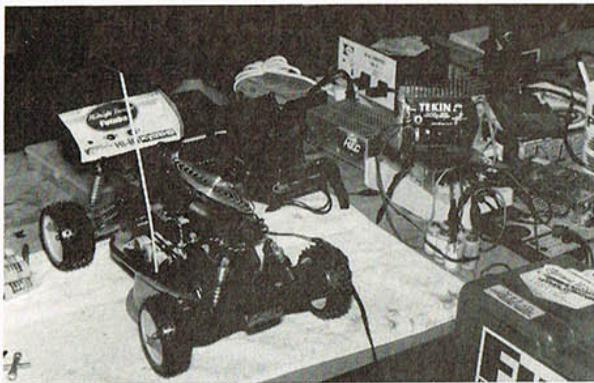
Cooling batteries while on charge (an attempt to charge their Hong-Kong's competitors battery pack to its limit).
