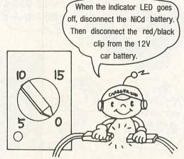
When the timer reaches zero and the indicator LED goes Off, recharging is completed. Disconnect the battery.
