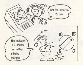
Turn the timer clockwise and set it to 15 min. The indicator LED will be on when the charger is charging.
