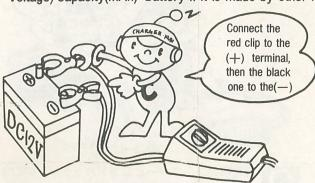
Connect the red(+) clip of the charger to the plus terminal of a 12V car battery, and black(-) clip to the minus, far away from battery. Don't run the car engine while charging battery.
