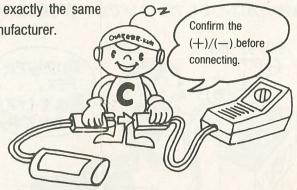
Connect the NiCd battery to the connector of the charger. \*Use "Battery-Charger Adapter" to recharge NiCd battery 7.2V-600mAh AE (for Motor Cycle). If the battery is only partially discharged, it is better to discharge completely before recharging in order to avoid over-charging. Don't recharge NiCd battery if it is still from use.
