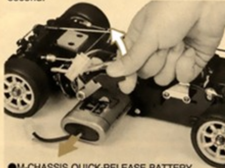
●M-CHASSIS QUICK-RELEASE BATTERY HOLDER (53238) Enables a quick battery replacement on Tamiya M-Chassis cars.
