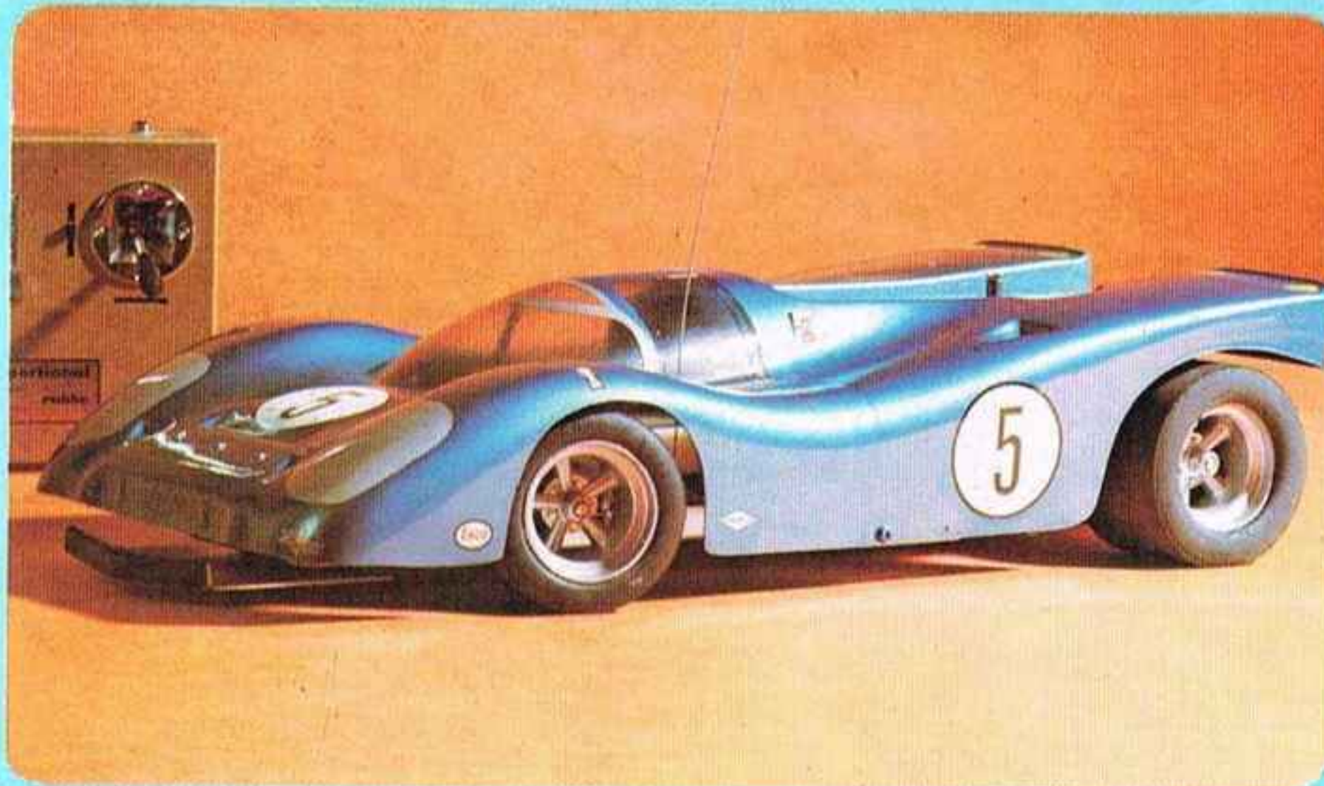
RC-CAR "K 1" Order No. 3300 Sports Car with choice of three bodies: Porsche 917: McLaren: Lola: Equipped with centrifugal clutch. 3 gear ratios available. 520 mm length.
