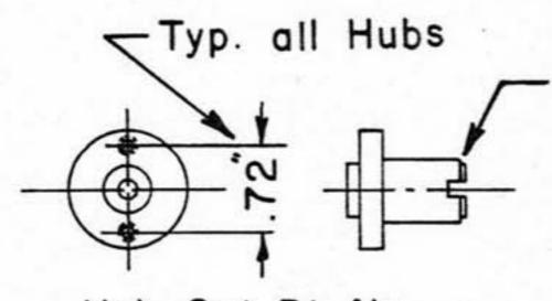
Tamiya Frog Hub shown, other Hubs have been designed to fit the axles of the appropriate cars. The wheel mounting holes are Typ. on all Hubs
