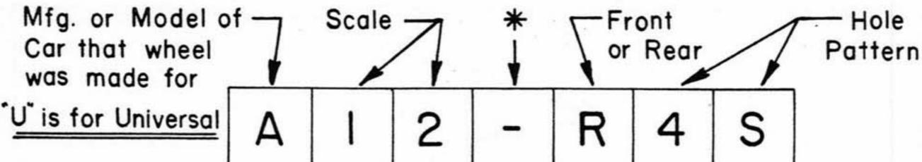
Example — Assoc. RC-12 (1/12 th Scale) — Rear Wheel with 4 Slot Pattern \* — This space used for special codes (such as 4 for 4 Wh. Drive)
