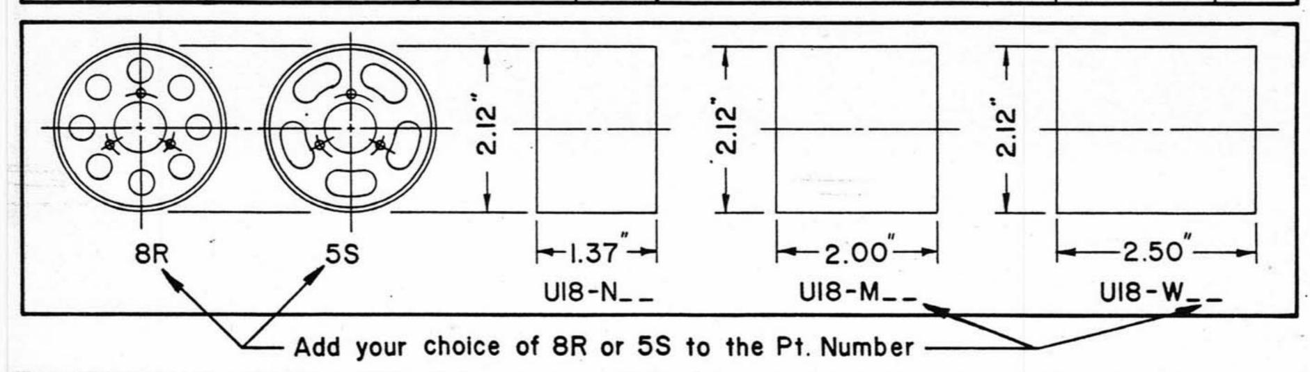
Assoc. RC500 (Plastic) Rear Wheels Modified for use with our Hubs.
